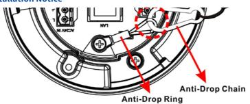
NOTE: For safety concern, it is recommended to hook up the camera with the anti-drop chain of the pendant when installing the camera. For more information about pendant and anti-drop chain, please contact the camera manufacturer.
